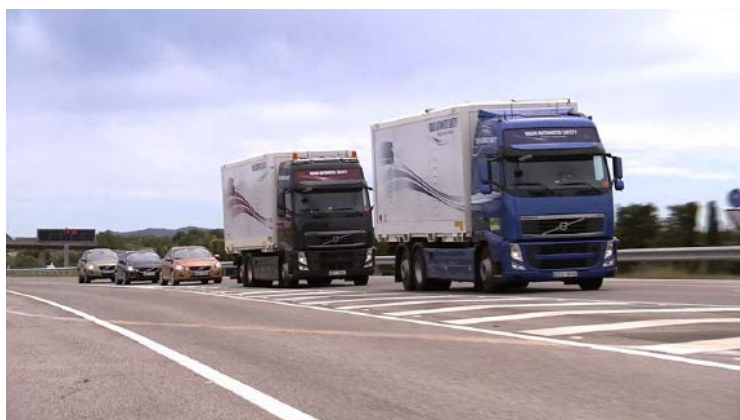
Figure 1: SARTRE's Road Train with 4 m (13 ft) Gaps and 90 km/h (56 mph) Speeds [28]
